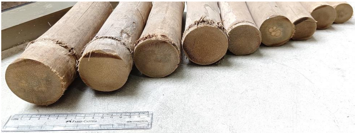
Figure 2. Raw material, D. stocksii , of various diameter from 60 to 20 mm (approx.) in natural form
